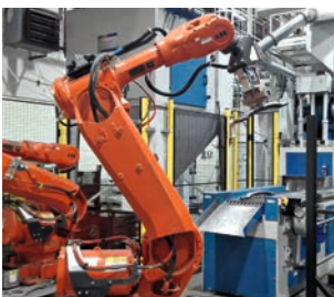
Robotic workplace equipped with robots for handling metal parts at high temperatures.
